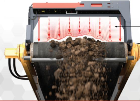
Secondly, the sensor measures the feed rate of the conveyor belt by an inductive sensor. Finally, by combining the cross profile and feed rate measurements, the resulting material data is readily available in cubic meters, yards or tonnes, and stored in the Sensor for easy download.
